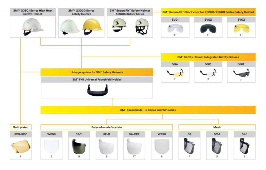
Impact performance B: Meets the requirement for protection against high speed particles for medium energy impacts (120m/s) F: Meets the requirement for protection against high speed particles for low energy impacts (45m/s) BT: Meets B as above. In addition meets this requirement after conditioning at 55°C and -5°C FT: Meets F as above. In addition meets this requirement after conditioning at 55°C and -5°C S: Increased robustness
